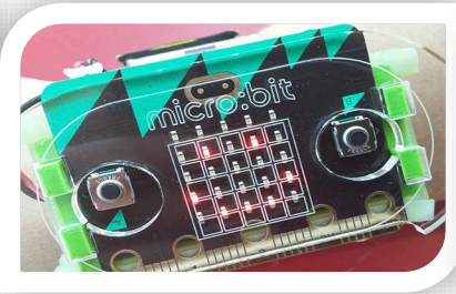
Microbit Step Counter
